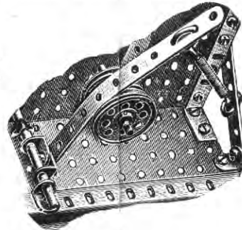
F —Spring Controlled Band Friction Brake.
