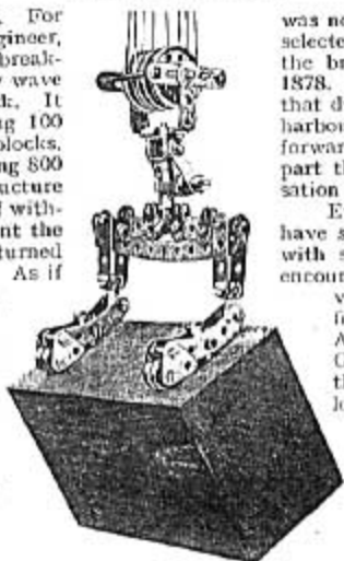
(Top) Concrete block held in position by Fidler's Gear. (Bottom) Meccano model of Fidler's Gear, which reproduces all the movements of the original
