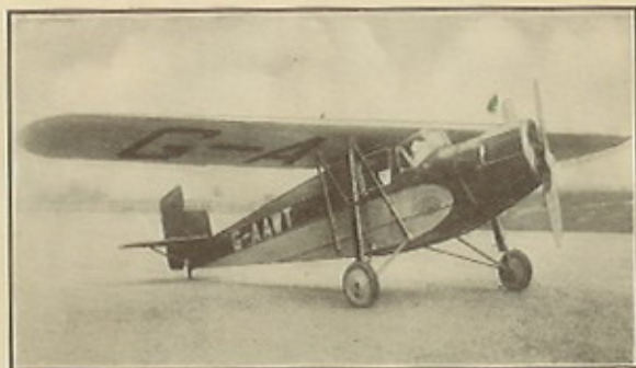
The Desoutter monoplane fitted with "Cirrus Hermes" engine. This machine has numerous excellent flights to its credit.
