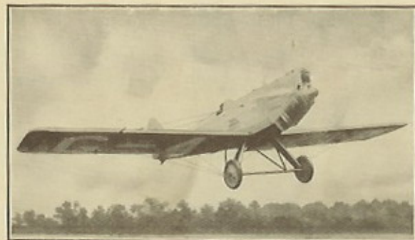
An Avro Avian Monoplane landing. This is a monoplane of the low wing type.
