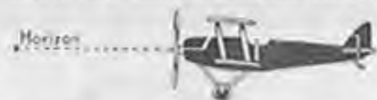
When the central column or "joy-stick" is vertical, the elevators are horizontal, and the machine flies parallel with the ground.
