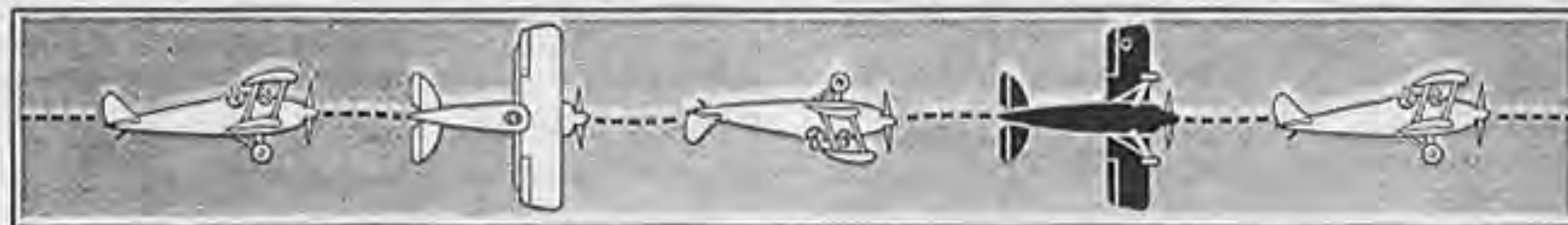
This sketch illustrates the various positions into which an aeroplane goes in course of one complete roll.
