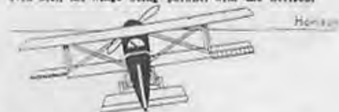
When the joy-stick is vertical the machine flies on an even keel, the wings being parallel with the horizon.
