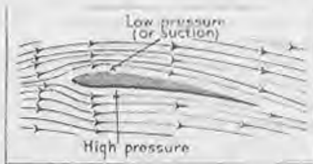
How air flows round an aeroplane wing.
