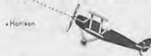
When the stick is pulled back, the elevators are raised and the machine climbs.
