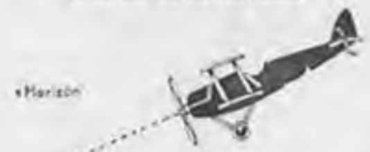
When the stick is pulled back, the elevators are raised and the machine climbs.
