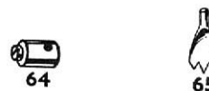
64. Threaded Boss 65. Centre Fork 69. Set Screw, 1/32" 69a. Grub Screw, 3/32" 69b. Grub Screw, 1/16" 69c. Grub Screw, 1/8"
