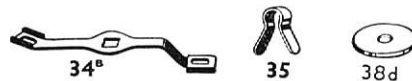
34b. Box Spanner 35. Spring Clip 36. Screwdriver 36a. Screwdriver (longer) 36c. Drift (for levering bolt holes into line) 37. Nut and Bolt, 3/32" 37a. Nut 37b. Bolt, 1/2" 38. Washer 38d. Washer, 3/8" 40. Hank of Cord
