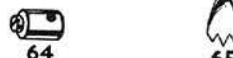
64. Threaded Boss 65. Centre Fork 69. Set Screw, 1/8" 69a. Grub Screw, 3/32" 69b. Grub Screw, 1/16" 69c. Grub Screw, 1/4"
