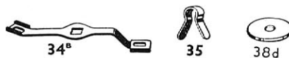
34b. Box Spanner 35. Spring Clip 36. Screwdriver 36a. Screwdriver (longer) 36c. Drift (for levering bolt holes into line) 37. Nut and Bolt, 3/8" 37a. Nut 37b. Bolt, 3/8" 38. Washer 38d. Washer, 3/8" 40. Hank of Cord
