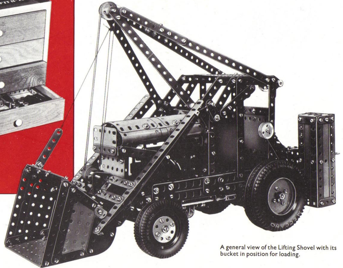
This striking model represents a popular type of mechanical lifting shovel used on large construction jobs where quantities of soil or other material have to be loaded into vehicles for removal from the site. Power is provided by a Meccano E15R Electric Motor that drives the road wheels through a differential. The lifting and unloading movements of the shovel are controlled from the cab, and the hoisting winch is fitted with an automatic brake.
